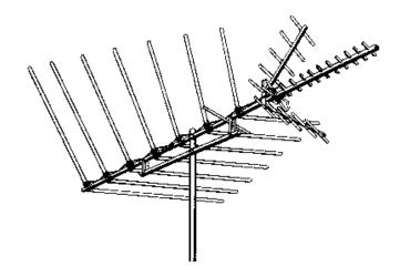
Pictured to the left is a picture of a Radio Shack VU-120 VHF/UHF Antenna. It consists of 7 VHF 3/2 Lambda elements, and a corner reflector UHF antenna. The UHF section has 10 director elements.
